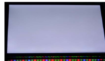
RGB Edge Lighting LED's for Flat Panel Illumination
