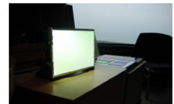
RGB Edge Lighting LED's for Flat Panel Illumination
